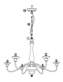
6.Connect the light fixture with canopy ③ with chain ①, let the wire go through the chain ② and canopy ③.
