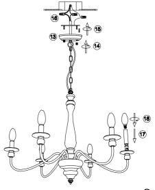
7.Install the bracket to the ceiling junction box with screw (§). 8.Connect the wire to your home line.
