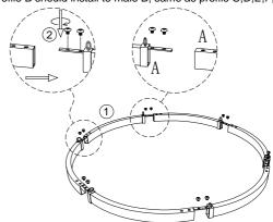
1. Assemble the split profiles ① to a completly ring, fasten the profiles with screw 2.
