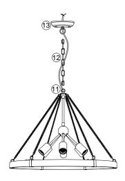
5. Hange the light fixture to the canopy ③ with big chain ②, let the wire go through chain @ and canopy 3.
