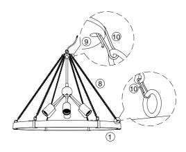
4. Hang the ring frame ① to the round plate of light fixture with hook  ${\small \circledR}$  of small chain  ${\small \circledcirc}.$
