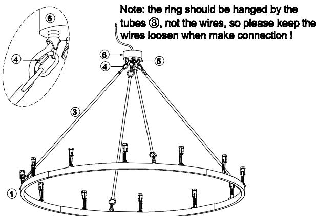
2. Let the wire go through the connected tube ③, hang the ring ① to the junction box ⑥ with carabiner hook screw connection ④, let the wire go through the junction box ⑥.
