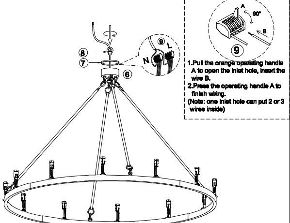
3. Connect all the wires by parallel with splicing connector ⑨ (all live line-L use one connector, and neutral Line-N use another connector).
