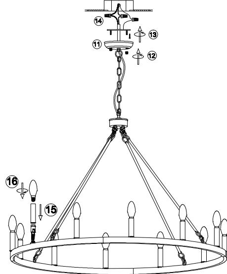
6. Install the bracket to the ceiling junction box with screw ⑬.
