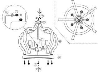
2.Install the wooden profile ③ to the round plate ② with screw ⑦, after that install the profile ⑥ to the round metal ring ⑨ with end cap screw 8. (when install the wooden profile⑥, please do not overexert to demage the profile)
