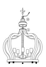
4.Let the wire go through the top cover  $\circledR,$  rotate the ring to fix the cover  $\circledR$  to the fixture.
