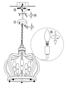
6.Install the bracket to the ceiling junction box with screw ①.
