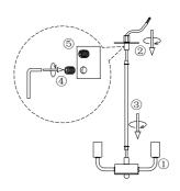
1.Let the wire go through the hanging tube ③ and round plate ②, rotate to fix them on the light fixture ① and lock it with grub screw ⑤ (by rotate hex key ④).
