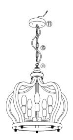
5.Hang the fixture 1 to the canopy 1 with chain 3, let the wire go through chain 3 and canopy 1.
