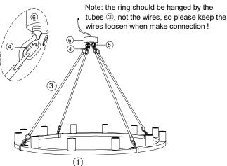
2.Let the wire go through the connected tube  $\, \Im$ , hang the ring  $\, \Im$  to the junction box  $\, \mathop{\textcircled{in}}$  with carabiner hook screw connection  $\, \mathop{\textcircled{4}}$ , let the wire go through the junction box  $\, \mathop{\textcircled{6}}$ .
