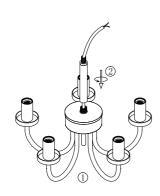
1. Let the wire go through the short hanging tube @, rotate the tube @ to fix on the threaded rod of fixture @.
