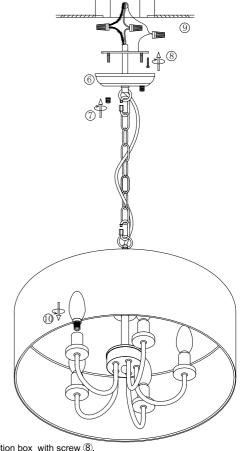
4.Install the bracket to the ceiling junction box with screw  $\ensuremath{\mathfrak{B}}.$
