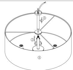
2. Let the wire go through the lampshade 4 and long hanging tube 3, rotate the tube 3 to fix lampshade together.
