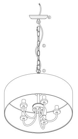
3. Hang the light fixture to the canopy  $\circledR$  with chain  $\noexpand$ 5, let the wire go through the chain  $\backsim$ 5 and canopy  $\circledR$ 6.
