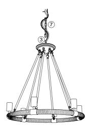
5.Install the chain  $\bigcirc$  to the fixture, let the wire go through the chain  $\bigcirc$ .
