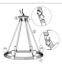
4.Hang the fixture  $\ensuremath{\mathbb{1}}$  to the connected box  $\ensuremath{\mathbb{5}}$  with the hooks of tubes  $\ensuremath{\mathbb{2}}.$
