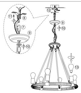
6.Install the bracket to the ceiling junction box with screw ①.7.Let the chain ⑦, main wire and the ground wire go through the ring ⑩, canopy ⑨ and bracket, hang the chain ⑦ to the bracket ⑧.
