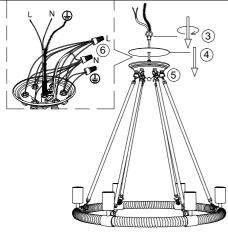
2.Connect all the wires by parallel with connectors ⑥(all live line-L use one connector, and neutral Line-N use another connector, ground line to round line).
