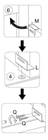
First, attach the upper end of door 14, then secure the lower end. Insert M into the slot, insert L and lock L with Q.
