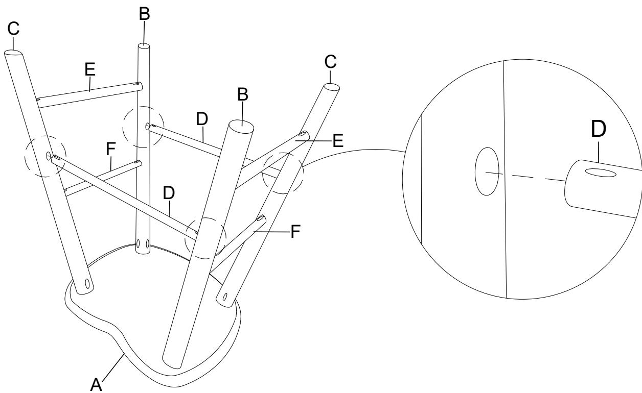
Step 5 . Tighten long stretchers (part D) and legs (parts B & C) using screws (part #1) and phillips head screwdriver.
