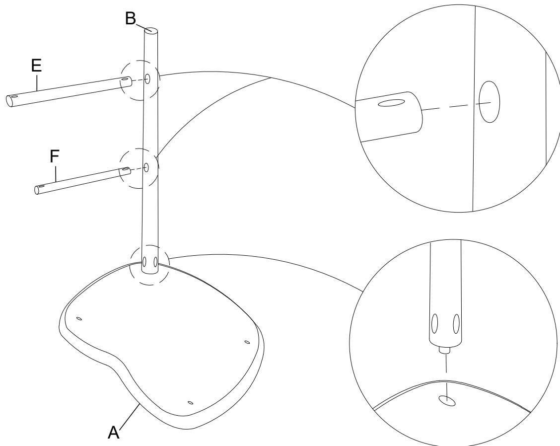
Step 2 . Attach leg (part C) to seat panel (part A) and insert medium stretcher (part E) and short stretcher (part F) into leg (part C). Tighten stretchers (parts E & F) using screws (part #1) and phillips head screwdriver.
