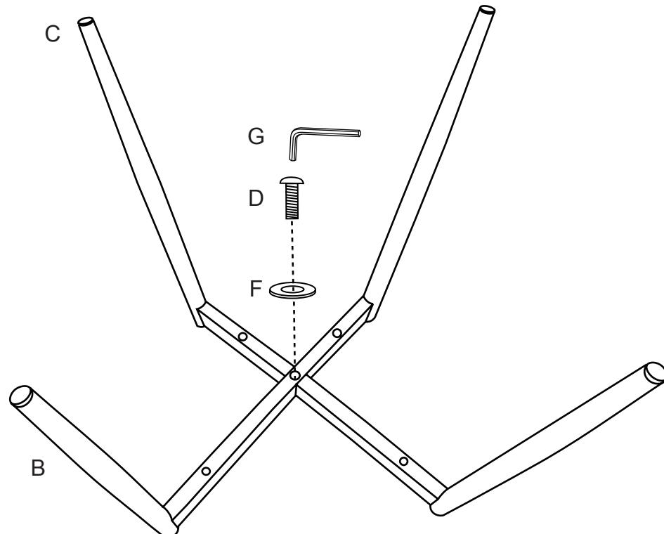
**STEP 2** Attach the Legs (B&C) to the Seat (A) by using Flat Washer (F), Allen Bolt (E) and Allen Key (G). Please tighten the bolts to 90%.
