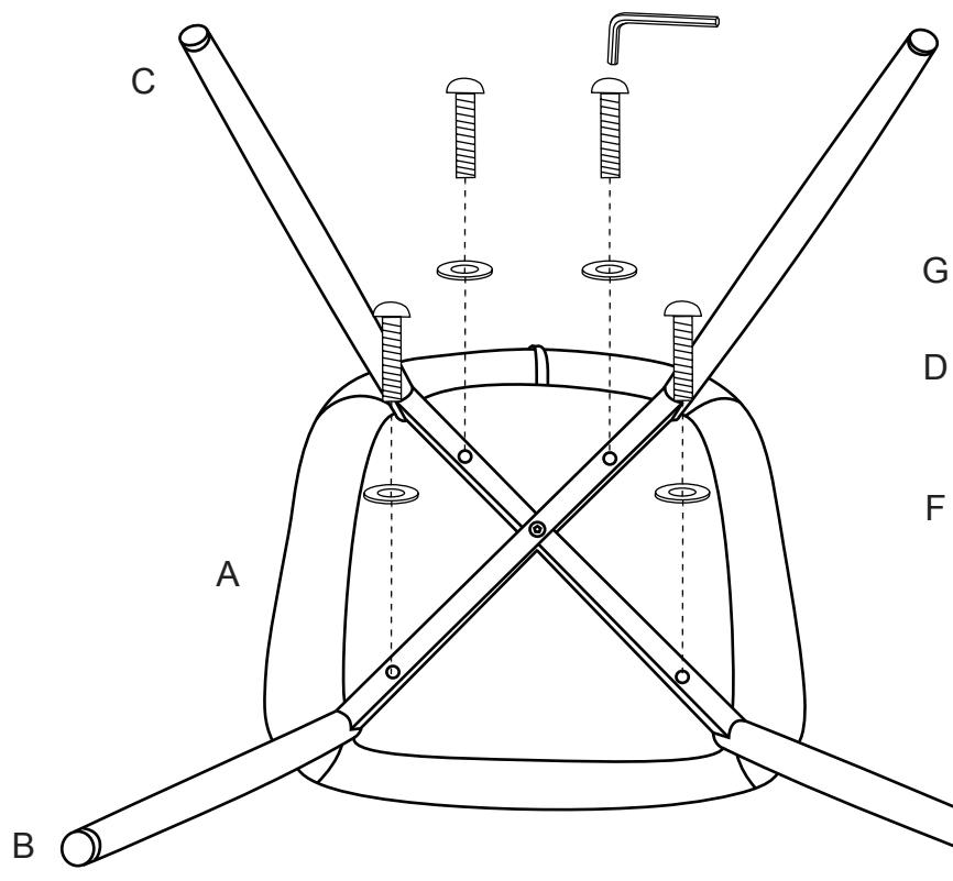
**STEP 3** Use body weight to adjust balance of chair, then tighten all the bolts 100%.
