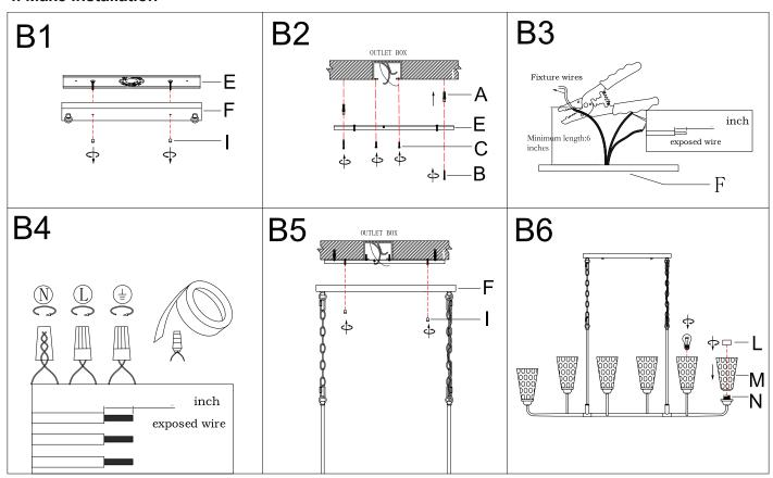
Step B1 » Unscrew knob nuts (I) and carefully remove mounting plate (E).
