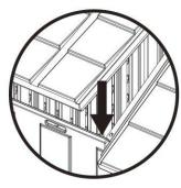
Tilt D2 into place, find the corresponding position and put it down.
