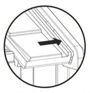
D1 and D3 are placed in the grooves of the iron frame, aligned with the grooves of the DL DR respectively and pushed forward.
