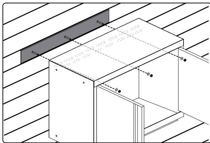
**Note:**For Locker cabinet attach second bracket 66" below first bracket.
