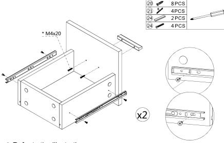
• Refer to the illustration, Apply Screws to fix the slides on the boards #11, #12.Use 24 Screws to install the handle.
