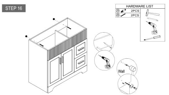
• Refer to the illustration, Draw the spacing between the walls on the cabinet, punch holes in the wall, and fix the cabinet to the wall with screws.
