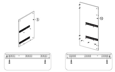
• Refer to the illustration to fix the Slide rails to the board #5 and #10 with screws.
