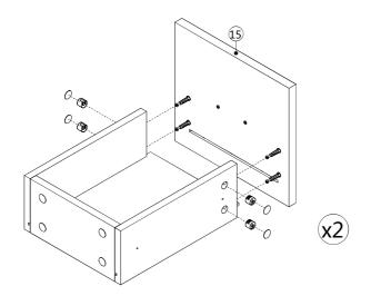
• Refer to the illustration, Draw the panel #15is inserted into the prepared plate, Then tighten the cam lock with the cover.
