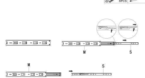
• Keep pressing here, then pull out to devide the slide.
