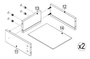
• Refer to the illustration, Connect the side plate #11, #12 with the back plate #13 with screws. Then insert the plate #14 in to the finished shelf.
