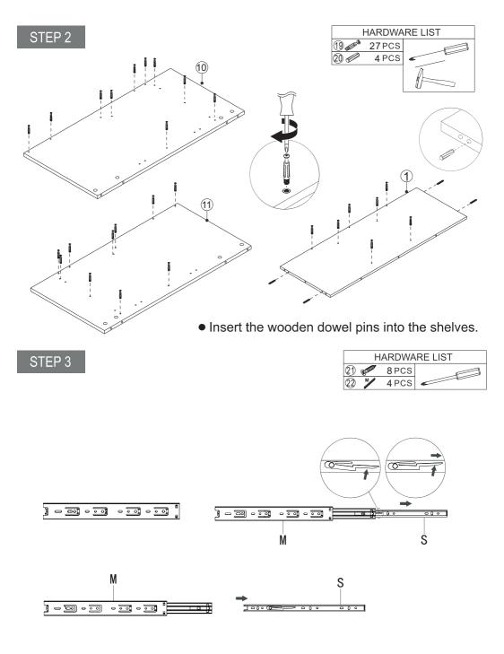
• Keep pressing here,then pull out to devide the slide.
