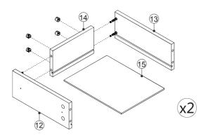
• Refer to the illustration, Connect the side plate #12, #13 with the back plate #14 with screws. Then insert the plate #15 in to the finished shelf.
