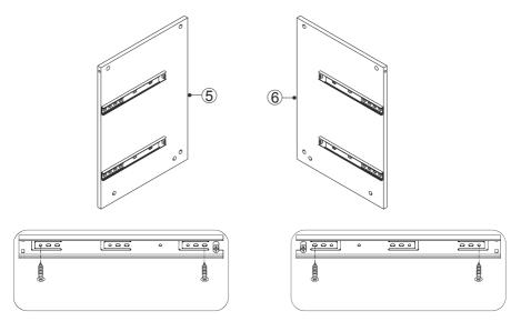
• Refer to the illustration to fix the Slide rails to the board #5 and #6 with screws.
