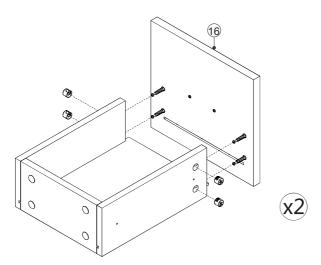
• Refer to the illustration, Draw the panel # 16 is inserted into the prepared plate, Then tighten the cam lock with the cover.
