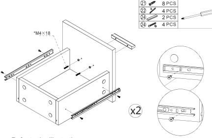
• Refer to the illustration, Apply Screws to fix the slides on the boards #12, #13. Use 24 Screws to install the handle.
