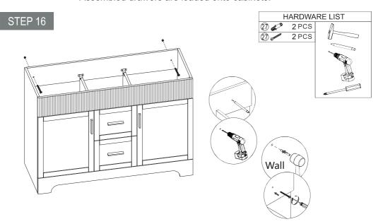
• Refer to the illustration, Draw the spacing between the walls on the cabinet, punch holes in the wall, and fix the cabinet to the wall with screws.
