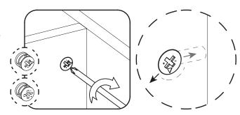
Still having issues? If a cam lock seems to be spinning in place or is not "catching" or pulling the panels together as expected, first remove the cam lock & try again while making sure that everything is properly positoned & oriented.
