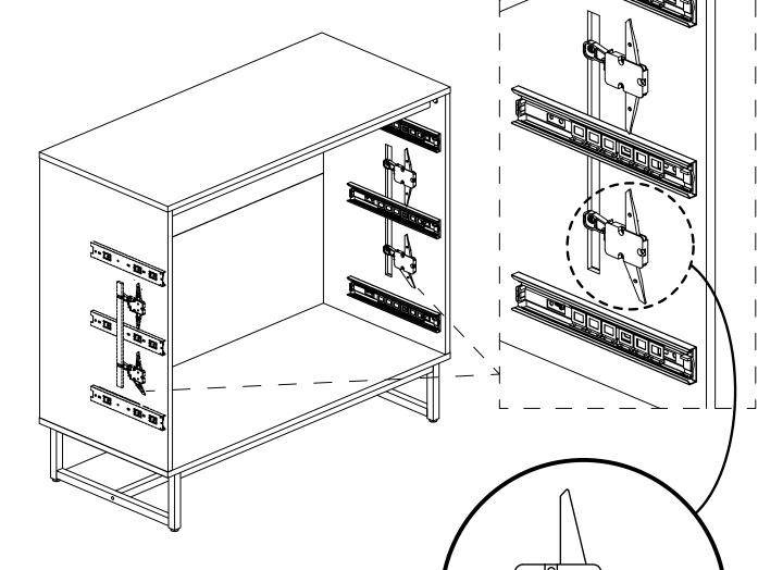
Important Note: As shown in detail on this page, you must place the bottom levers of the bottom safety mechanisms in the forward position when installing the bottom drawer.
