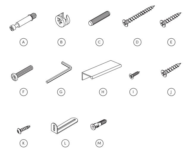
Alright, let's get this thing fired up! Using the ¼"\*30mm Bolts (F), connect the Metal Side Frames (10) to the Top Metal Stretchers (8) and Bottom Metal Stretcher (9). Tighten bolts to 75% using the Allen Key (G).
