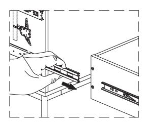
**STEP 2:** Begin to align the rails on the sides of the drawer with the inner ball bearing slides that are being held in place.
