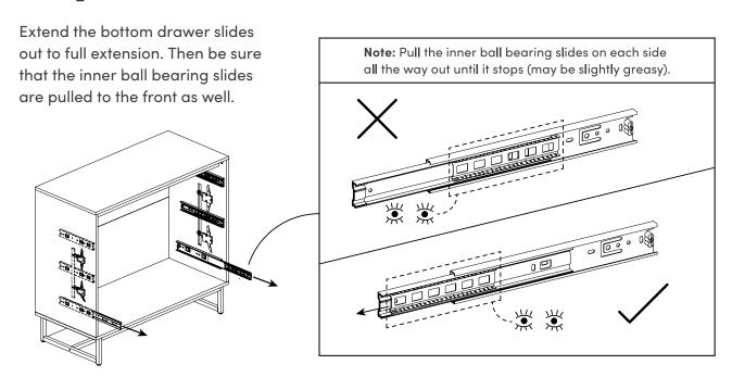
Install the bottom drawer onto the extended bottom slides.
