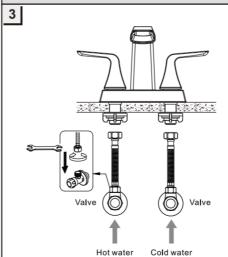
3. Connect the inlet hose as shown, take note of the "Red" & "Blue" index from the handle, "Red" for connecting to the valve for supply hot water, and "Blue" for connecting to the valve for supply cold water.
