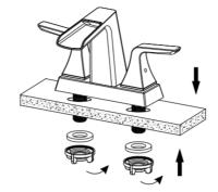
1.Please confirm the two holes on the basin are through holes as shown from the instructions before install. First, remove all fixing sets from the fixed group, and then put the body through the hole on the basin, assemble all fixing sets to the body.
