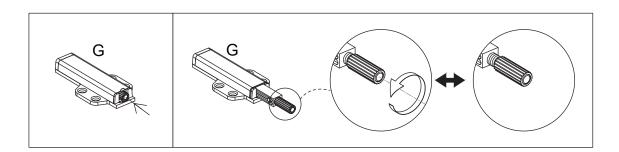
If the drawer cannot be automatically popped out after installation, adjust the length of G device as shown in the figure.
