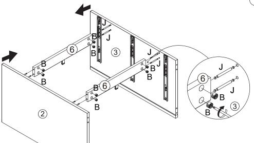
Do not use an electric screwdriver, do not use force during the rotation of the accessories, otherwise it may cause the board to crack.
