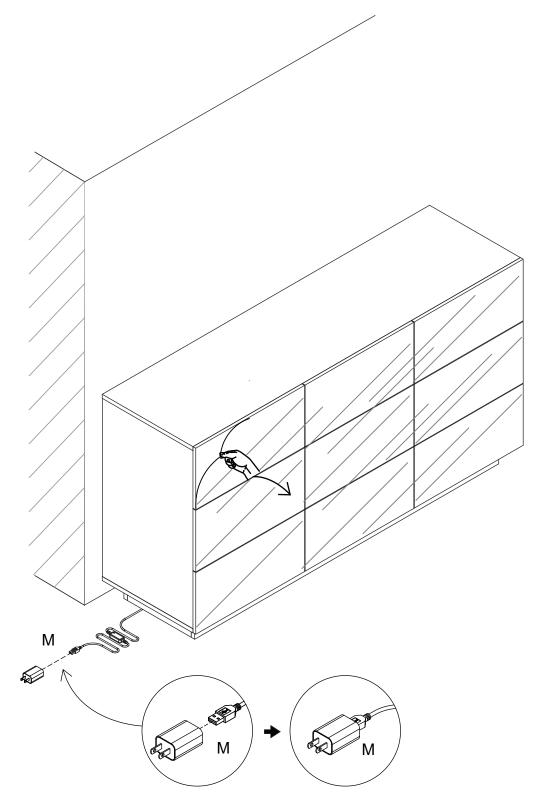
Connect the cable to the light strip.
