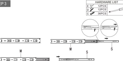
• Keep pressing here, then pull out to devide the slide.
