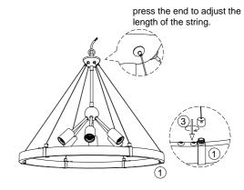
4.Rotate to install the end cap 4 on the thread rod of the ring 1, adjust the height of the string.
