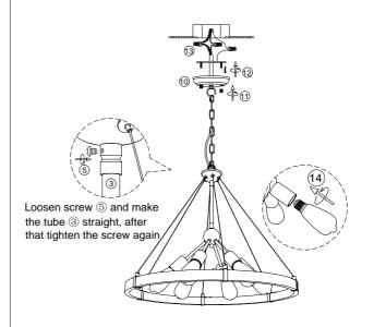
6.Install the bracket to the ceiling junction box with screw 1.
