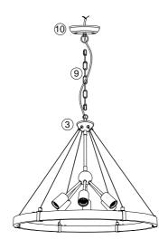
5.Connect the fixture ③ to the canopy ⑩ with chain ⑨, let the wire go through the chain ⑨ and canopy ⑩.
