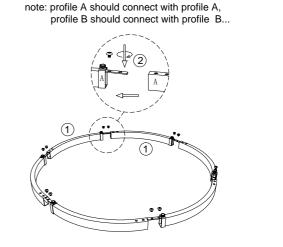
1.Install the profile 1 to a ring, and lock it with screw 2.
