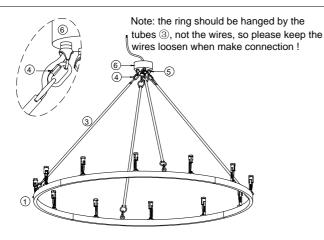
2.Let the wire go through the connected tube 3, hang the ring 1 to the junction box 6 with carabiner hook screw connection 4, let the wire go through the junction box 6.
