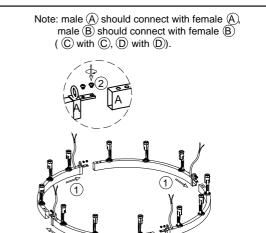
1. Assembled the split parts 1 to a completely ring fixture like picture showed, pushed the split parts and fix with bolt screw 2.
