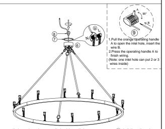
3.Connect all the wires by parallel with splicing connector (9) (all live line-L use one connector, and neutral Line-N use another connector).
