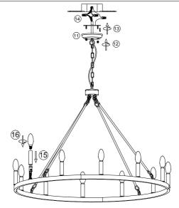
6.Install the bracket to the ceiling junction box with screw ③.
