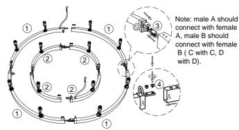
1.Assemble the big ring ①, firstly install the male and female connector ③, make sure the connector ③ tighten enough can not pull out anymore, and then put the split parts together, lock it with screw ④.(same step to install the small ring ②.)
