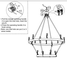
4.Let the wires go through junction box ③ and connect all the wires by parallel with connectors ⑫(all live line-L use one connector, and neutral Line-N use another connector).
