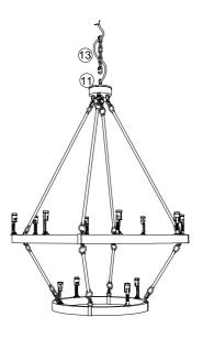
6.Install the chain  $\ensuremath{\mathfrak{B}}$  to the fixture, let the wire go through the chain  $\ensuremath{\mathfrak{B}}.$
