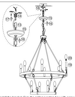
7.Install the bracket (4) to the ceiling junction box with screw (1).
