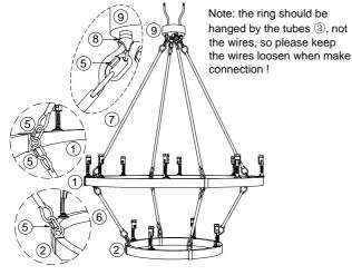
2.Let the wire of small ring @ go through the short hanging tube @, hang the small ring @ to the big ring @ with hanging tube @.(Note: the wires of two rings can not meet at the same side.)
