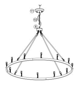
5.Connect the canopy ① and the light fixture ⑧ with chain ⑩.
