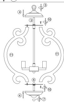
3. Install the wood profiles ① to the top plate ② and down plate ⑥ with screw ⑩, fixed the cover ④ to the plate ③ with hanging ring ⑤, fixed the cover ④ to the down plate ⑥ with end cap ⑦.(Do not overexert when rotating the screw ⑩, lest breaking off the wood profile①, adjust the profile to right position like picture showed after installation.)
