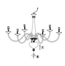
2. Install the bottom box ⑦ to the fixture ① with end cap ⑧.
