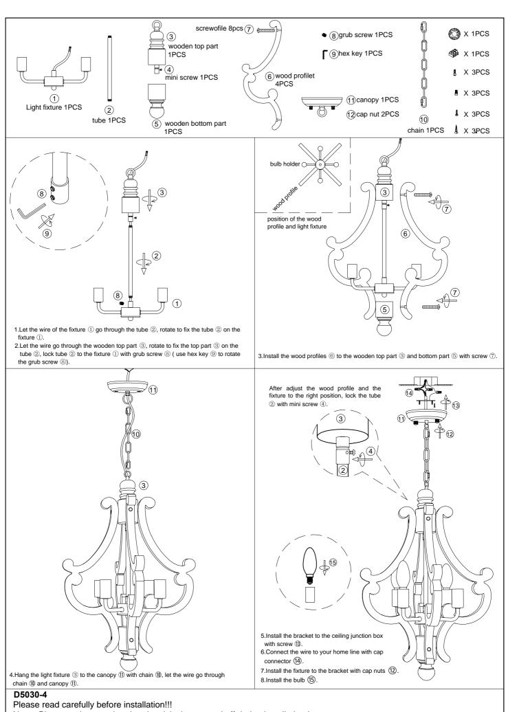
Note: Please make sure that the electricity is powered off during installation!
