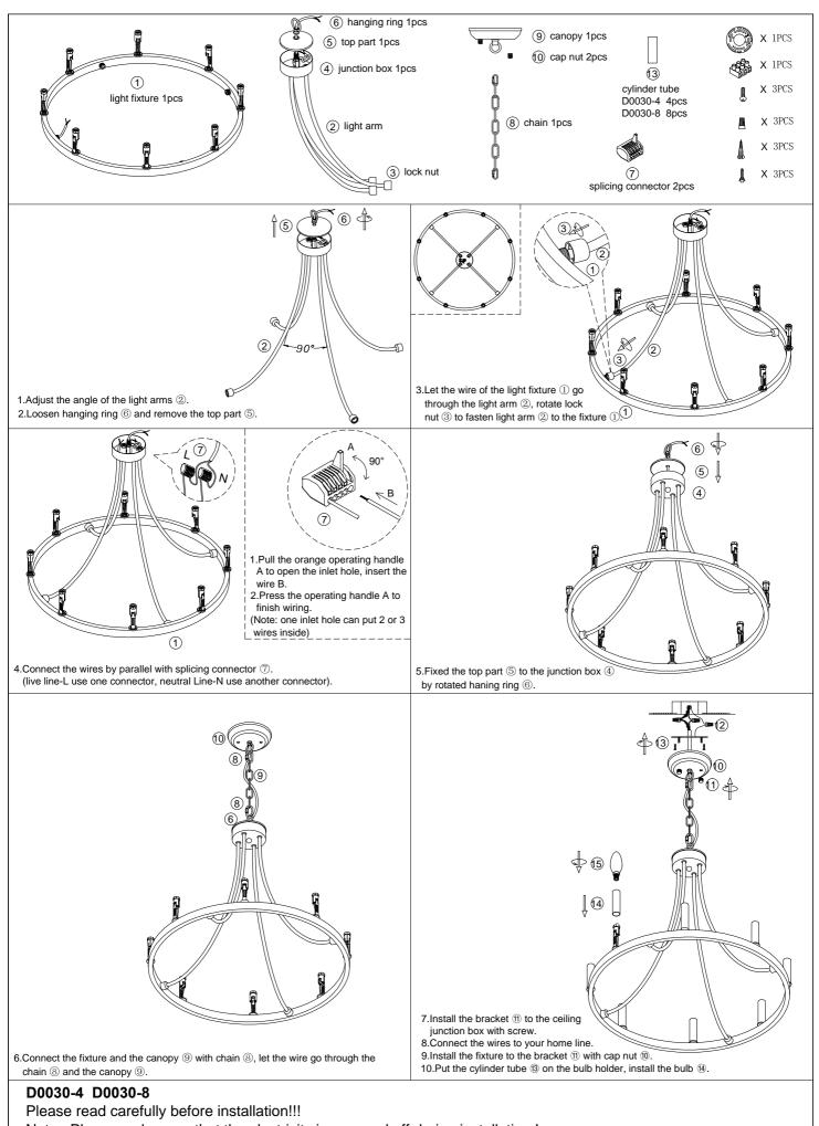
Note: Please make sure that the electricity is powered off during installation!
