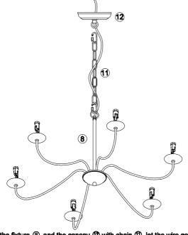
5.Connect the fixture (a) and the canopy (b) with chain (b), let the wire go through the chain (b).
