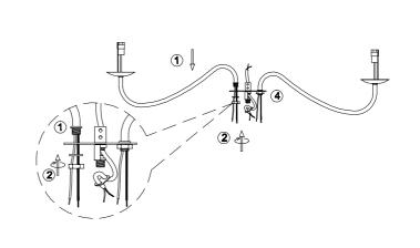
1.Install the arms 1 on the plate 3 with lock nut & teeth lock washer 2.
