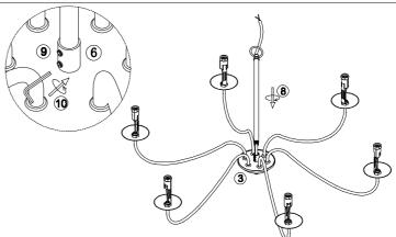
4.Let the wire go through the hanging tube (a), rotate to fasten the tube (a) to the connect tube (b), lock the tube (a) with grub screw (b) by rotate hex key (b).
