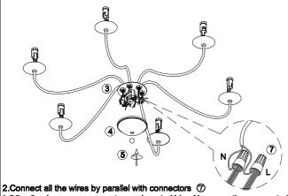
2.Connect all the wires by parallel with connectors (7)
