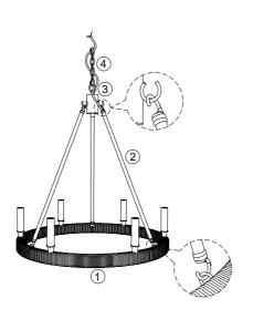
3.Connect the light fixture 1 and the hanging part 3 with tubes 2, let the wire go through ring of part 3 and chain 4.
