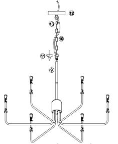
5.Let the wire go through the ring ① of the chain ⑩, rotate the ring ① to fix chain ⑩ to the fixture, connect the chain ⑩ to the canopy ② by carabiner hook screw connection ③, let the wire go through the chain ⑩ and canopy ②.
