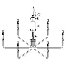
3.Install the cover 6 and the tube 6 on the bottom plate 9 with thread rod 7.
