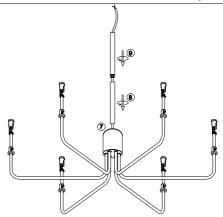
4.Let the wire go through the tube 8 and tube 9, rotate to fix two tubes on thread rod 7.
