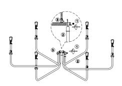
1.Install the arms ② to the bottom plate ③ by grub screw ③, and adjust the arms to the right position.
