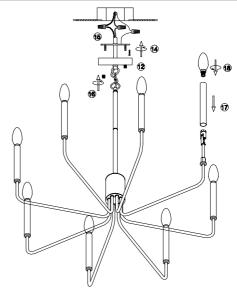
5.Install the bracket (9) to the ceiling junction box.
