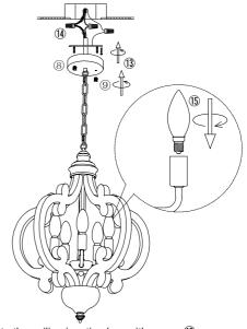
5.Install the bracket to the ceiling junction box with screw (3).6.Connect the wire to your home line with cap connector (4).7.Install the light fixture to the bracket with cap nuts (9).8.Install the bulb (5).
