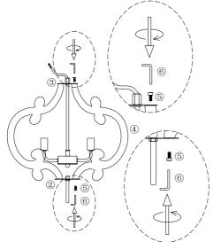
2.Install the wooden profile ④ from the hole of tube ③ to the hole of plate ② with screw ⑤. (after installed the wooden profiles, adjust to the suitable position, the screw should not be too tight to avoid damaging the wooden profile.)
