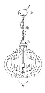
4.Hang the fixture to the canopy 8 with chain 1, let the wire go through the chain 1 and canopy 8.
