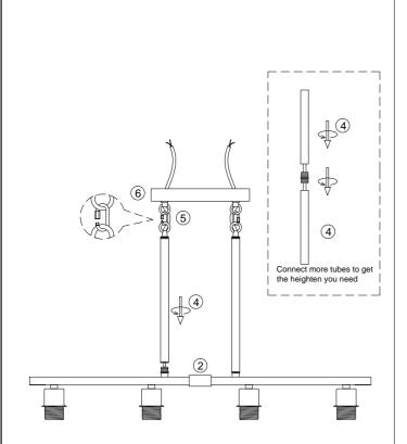
2.Let the wire go through the hanging tube4, rotae to fasten the tube on the fixture 2, connect the fixture and the canopy 6 with carabiner hook screw connection 5, after that let the wire go through canopy 5.
