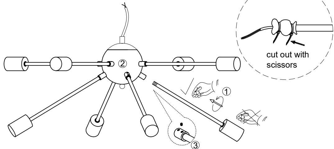
1. Turn and fix the tube1 on the ball2, lock it with screw3.
