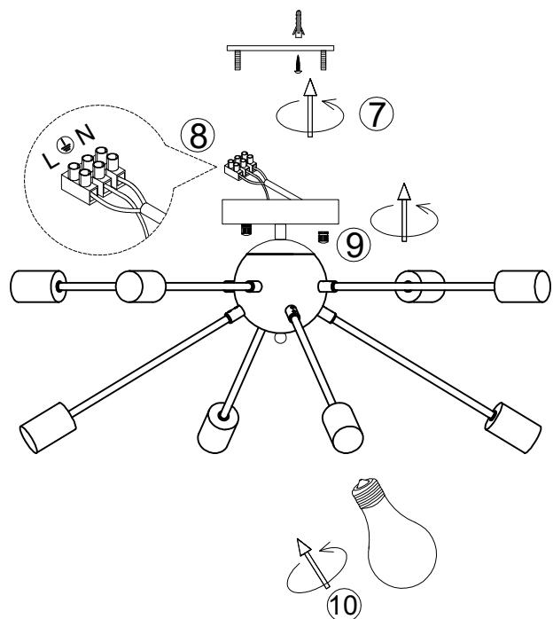
2. Rotate to install the thread rod 4 to the ball 2, fasten the canopy 6 and ground line to the ball with lock nut and teeth lock washer5.
