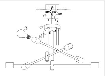
5.Install the bracket on the junction box with screw (11).
