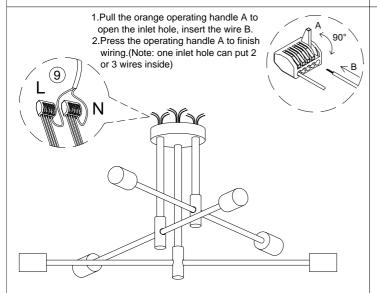
4.Connect all the wires by parallel with connectors <sup>(9)</sup> (all live line-L use one connector, and neutral Line-N use another connector).
