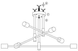
3.Install the hanging tube fixture 5 on the canopy 4 with screwing locknuts 6.
