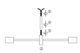
2.Let all wires go through the two heads threat rod ③, install the threat rod ③ on the middle tube, after that wire go through the hanging tube ⑤ and single head threat rod ⑥, connect the hanging tube and the single head threat rod with the fixture.
