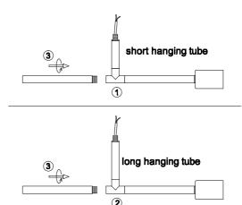
2.Rotate to install the tube ③ to the light arm.
