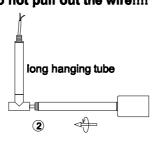
1. Rotate to install the light arm  $\, \textcircled{\scriptsize 1}$  &  $\mbox{\scriptsize 2}$  to the hanging tube.
