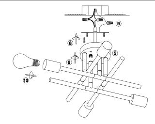
6.Install the bracket to the ceiling junction box with screw (a).
