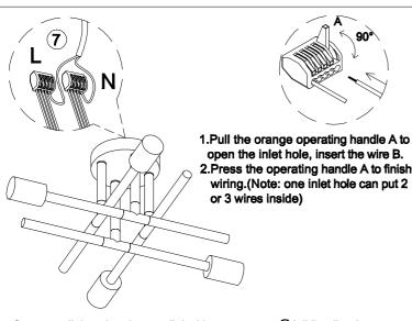
5.Connect all the wires by parallel with connectors ⑦(all live line-L use one connector, and neutral Line-N use another connector).
