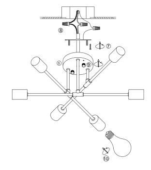
3.Install the bracket  $\ensuremath{{\mathbb T}}$  on the junction box with screw.
