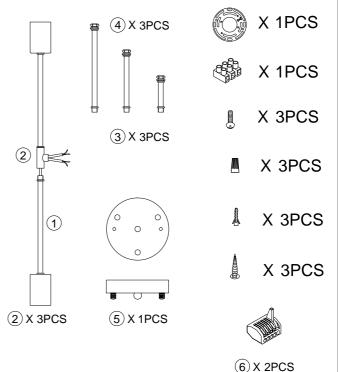
1.Install the light arm 1 with arm 2, after that let the wire go through the tube 3, turn to fix tube 3 on the light arm.
