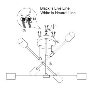
2.Install the light arm 3 to the canopy 5 with lock nut & teeth lock washer 4, after that connect the wires by parallel with splicing connector (all live line-L use one connector, and neutral Line-N use another connector).
