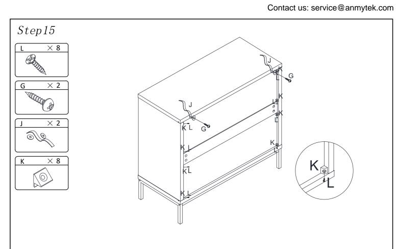
**Kindly note:**This is a very important step that can not be skipped. Please follow the step to screw the plastic pieces into the corner of the back panel tightly. If you forget to fix these pieces, it may result in the instability of the whole item.
