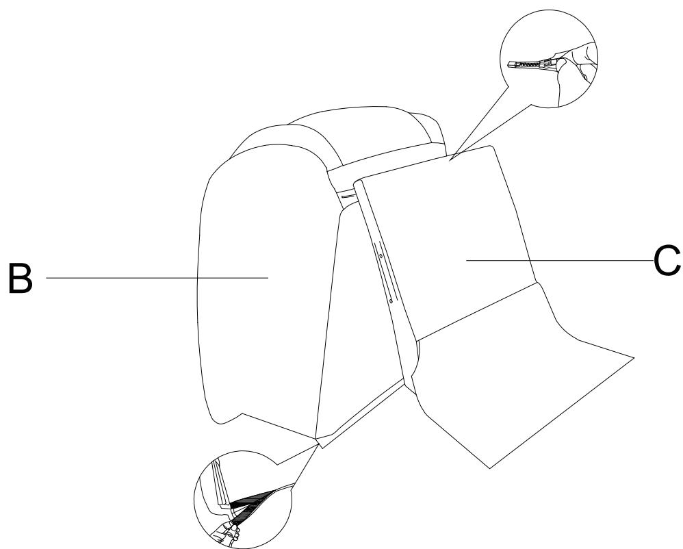
Step 3 Insert the arms into the seat in a way that they fit properly .
