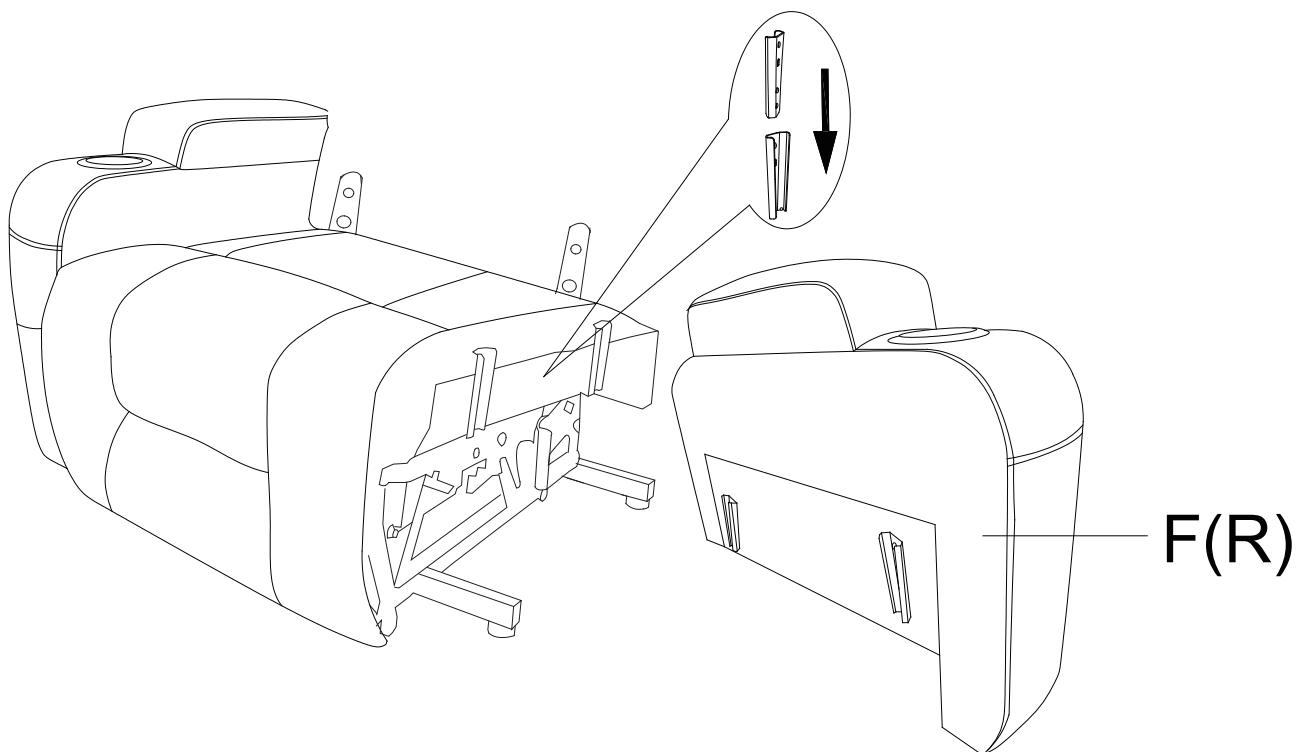
Step 5 Plug the back pad into the seat frame , then connect the massager lines: white with white , red with red , black with the power lines , connect the massage line with the hand controller.
