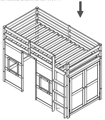
Make sure to tighten all the screws of the bed.
