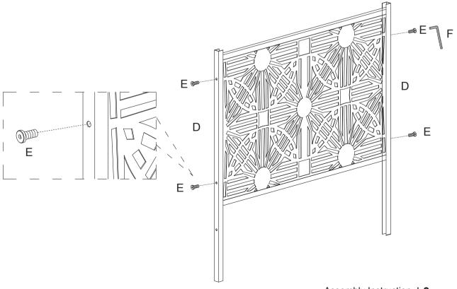
Attach the assembled part 2 onto the assembled part 1. Secure the two assembled STEP 5 parts using the remaining 2 Bolts (E) with the Allen Key (F).
