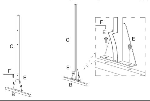
Slide the first Screen Panel (A) into the channel of the two assembled Bottom STEP 2 Long Stand Riser Bars (C), secure it using 2 Bolts (E) from each side with the Allen Key (F).
