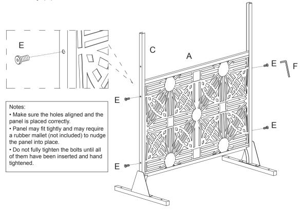
Slide the second Screen Panel (A) into the channel of the two assembled Bottom STEP 3 Long Stand Riser Bars (C), positioning it above the first screen panel. Secure it using 1 Bolt (E) from each side with the Allen Key (F). You now have the assembled part 1.
