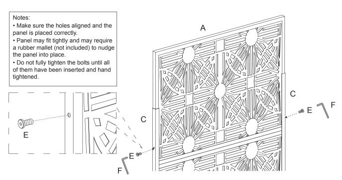
Attach the Top Short Support Bars (D) to the last Screen Panel (A). Secure it using STEP 4 2 Bolts (E) from each side. Make sure the holes aligned and the panel is placed correctly. Hand tighten only. You now have the assembled part 2.
