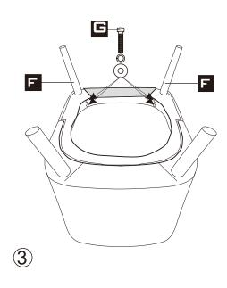
Put the screws in the holes, tight the screws, but not too tight,90% is ok
