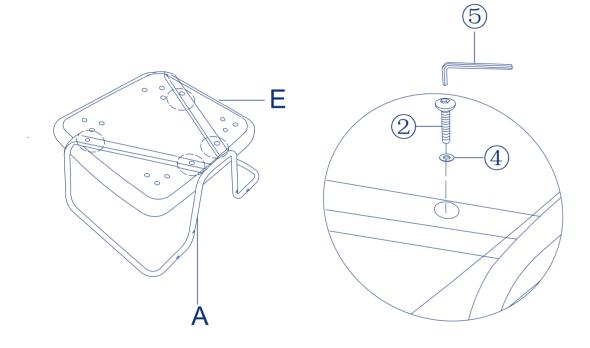
Leave bolts 80% tightened, tighten after all alignment.
