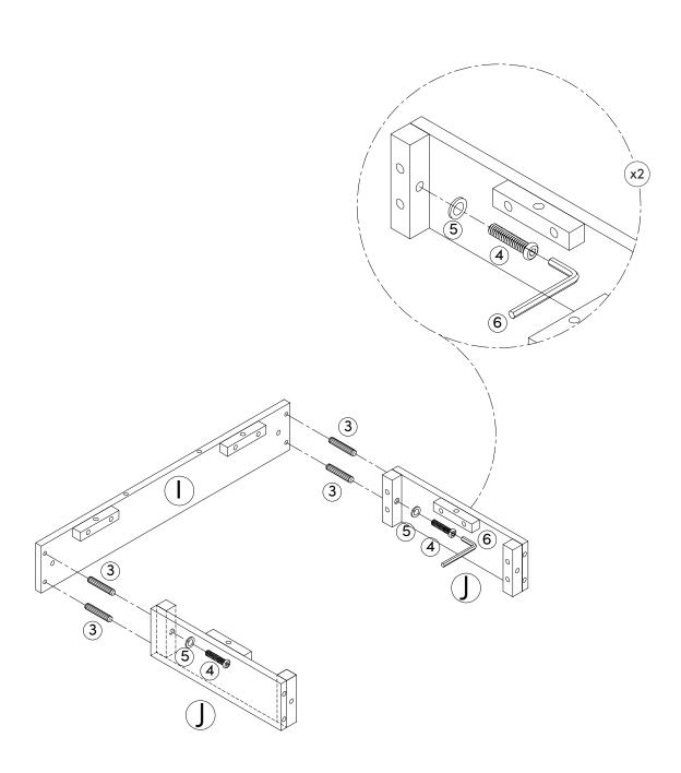
Next, set the pieces that you assembled in Step 9 into place on the Bottom Panel (F) by inserting & aligning the Wooden Dowels (3) in their respective pre-drilled holes.
