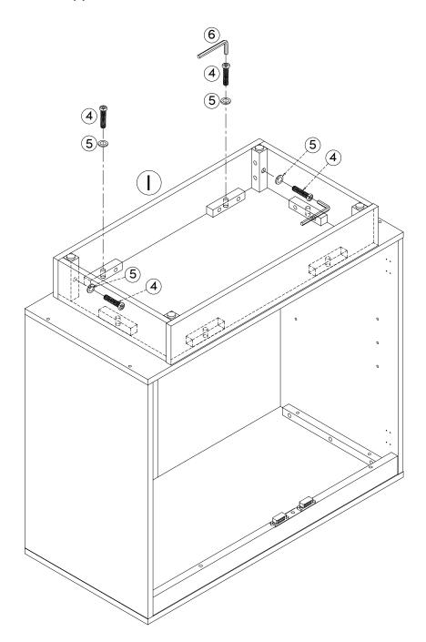
Once everything is lined up and partially secured, go ahead and re-tighten all previous connections to 100% tighten.
