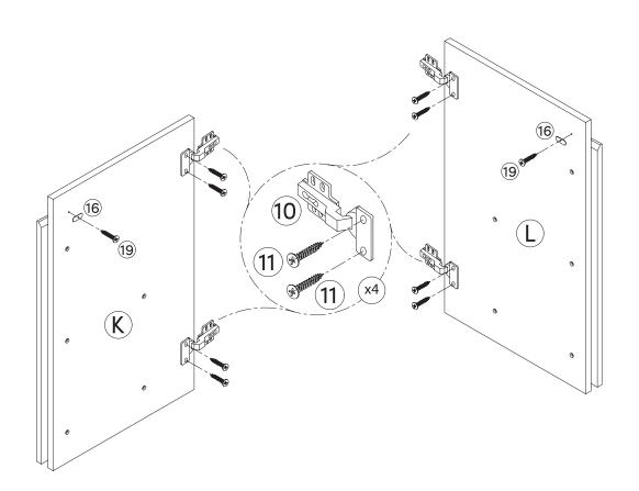
It's all coming together! Secure the doors to the unit by the Hinges using the M3.5\*15mm Screws (11).
