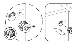
Using a screwdriver, you will turn the cam lock until it stops, usually between 130° or 180°. You will feel the panels pulling closer until they are secured.
