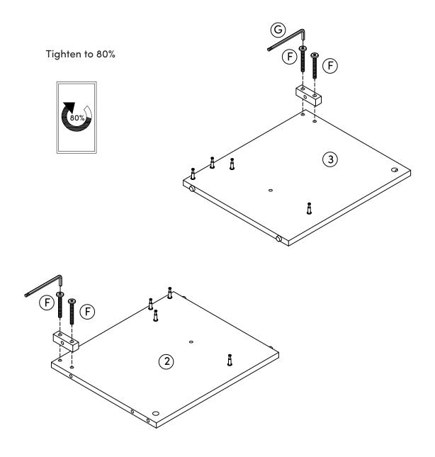
Almost there! Now, attach the Right Side Panel (3) to the assembly you've been working on. Use the Cam Locks (B) to secure the parts together. Reference the image below to make sure you insert the Cam Locks in the right order.
