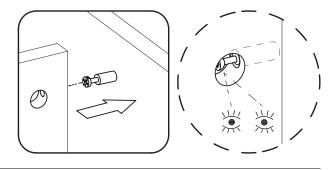
Next, you will notice the cam lock has a "C" shaped back. Commonly, an arrow on the front of the cam lock points in the same direction as the open section on back.
