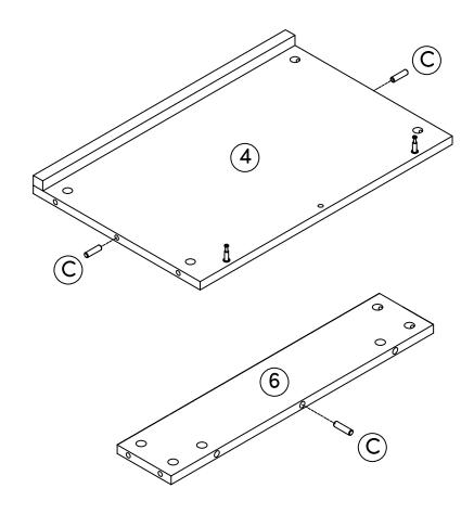
Let's get things moving! Take the Bottom Shelf Stretcher (6) and attach it to the Bottom Shelf (4) by pushing the pieces together. Ready for some tightening action? Use the Cam Locks (B) to secure everything in place.
