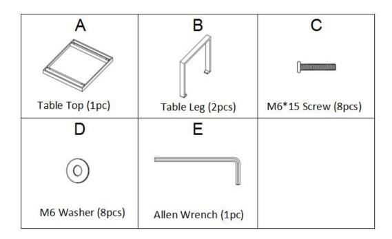
Secure table legs (B) to table top (A) by using 8 screws (C) and 8 washers (D) with allen wrench (E). Fully tighten all screws.
