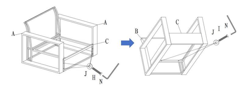
3. Secure Side Panels (D&E) to chair back (B) with 8 washers (J) and 8 screws (H) by using allen wrench (N). Do not tighten all screws now.
