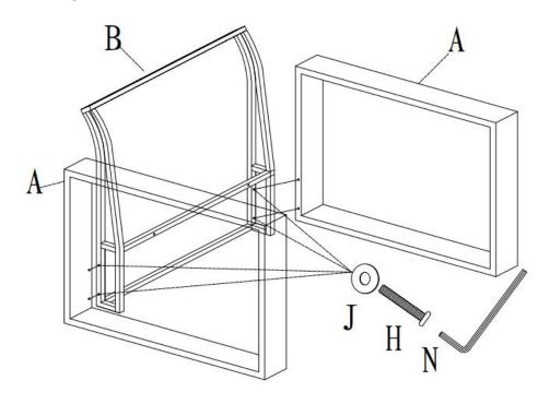
2. Secure chair seat (C) to chair arms (A) and chair back (B) with 6 washers (J) and 6 screws (H&I) by using allen wrench (N). Do not tighten all screws now.
