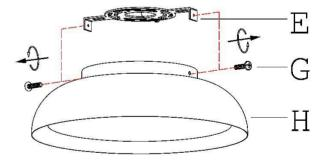
3 » Carefully pass the supply wires from the outlet box through mounting plate (E).
