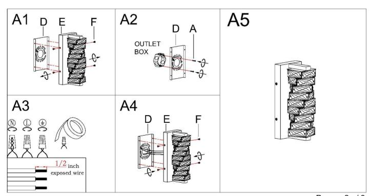
Step A1 » Unscrew screws (F) from back plate (E) then gently remove mounting plate (D). Then set them aside for later installation.
