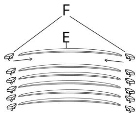
Make sure the convex surface like the bridge is upward and put on the caps
