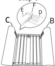
Press the cap to lock the slate in the hole (convex surface is still upward)
