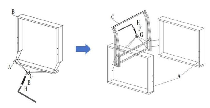
2. Secure chair seat (D) to chair arms (A) and chair back (C) with 10 washers (G) and 10 screws (F) by using allen wrench (H). Fully tighten all screws now.
